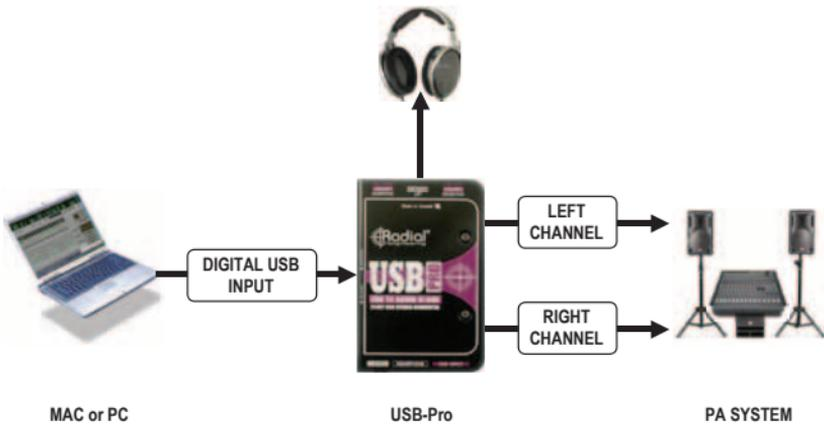
The USB-Pro is very easy to setup and use because it derives power from the USB connection and automatically configures the sampling rate and bit depth without the need for special drivers. The USB-Pro can be used for audio playback, system testing and for transferring digital audio files to analog for processing.
